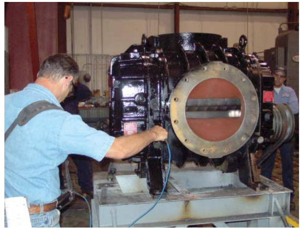
Testing a rebuilt blower.
